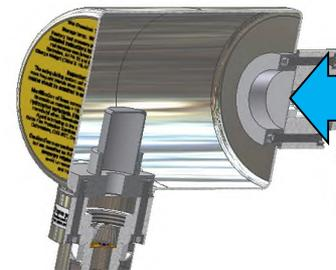
Burst disc at canister inlet breaks. Water flows into the canister.
